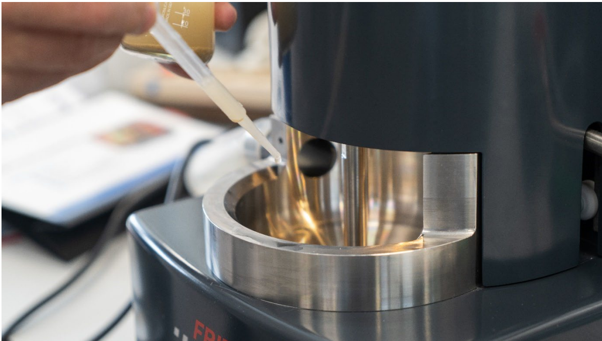
Fig. 2: Pipetting the pre-dispersed sample into the wet measuring unit of the A-22 NeXT
